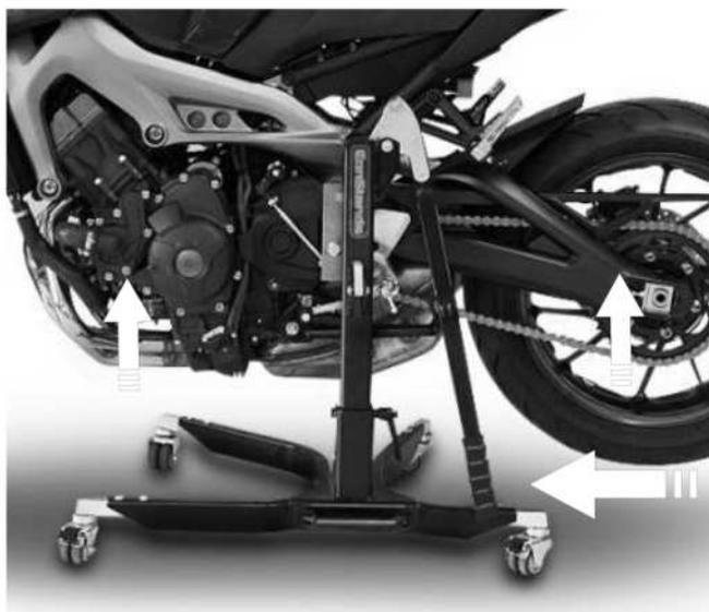
7. Press the lever arm of the central mounting stand so far down until the desired lift is reached.
