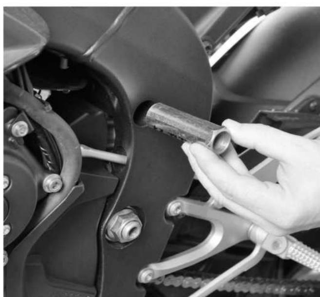
4. Install the supplied bushing into the frame hole. Attach it to 50 Nm.
