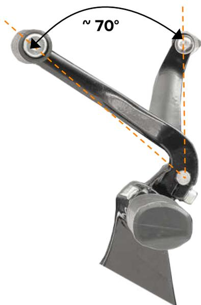
7. Mount the **shiftpeg (6)** on the **shift lever (5)**. Use the **shiftpegcrew (7)** and liquid threadlocker for this purpose.
