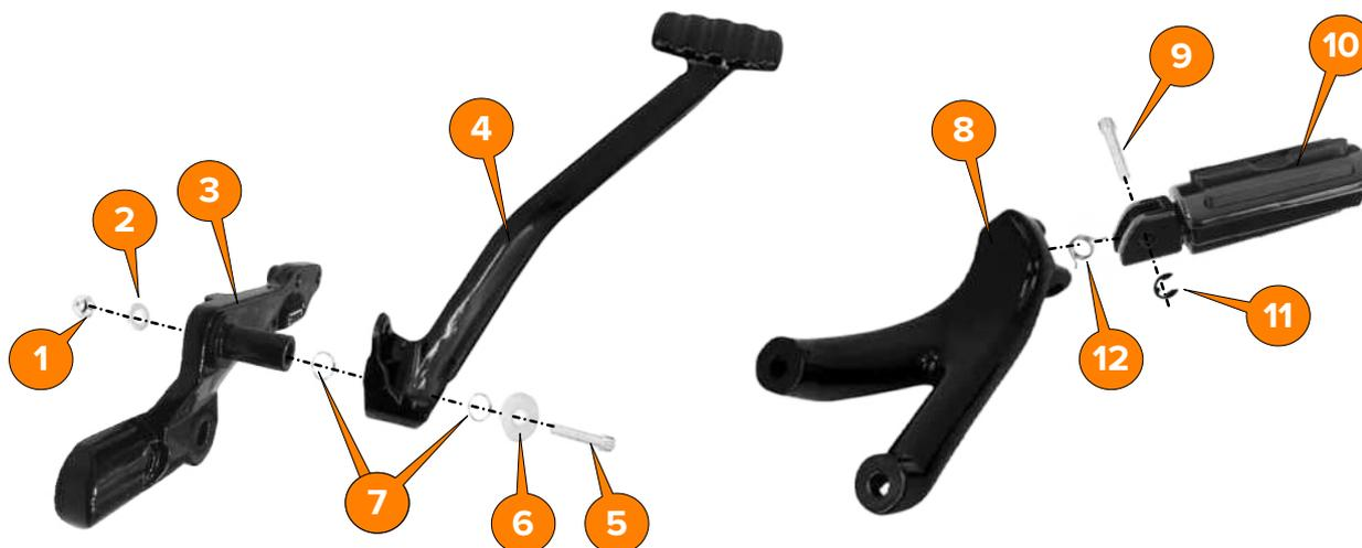
1. Fit the first **O-ring (7)** to the **brake pedal bracket (3)**.
