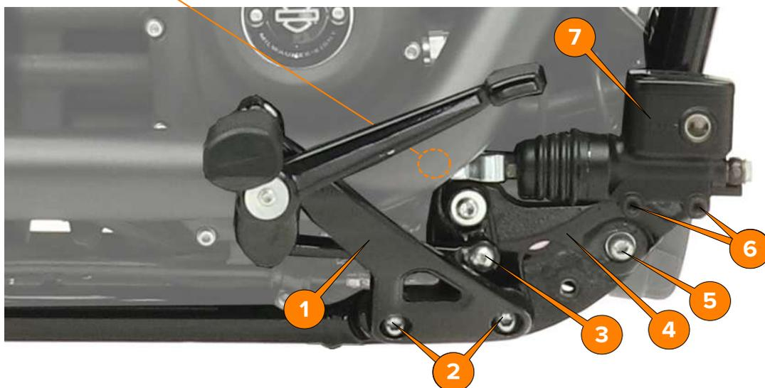
4. Loosen the **original screws (6)** and support the **rear brake master cylinder (7)**.
