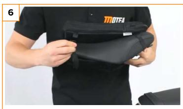
**Step 6:** Detach the seat from the vehicle, guide the fastening straps around the seat and insert them into the loops on the other side of the seat cushion.
